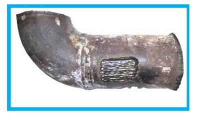
**Case History 1:** casehistoryinvolvingtheinstallationofatotalofsixCRV<sup>®</sup>s,oneupstreamofeachofsix2"extra heavy pipe elbows for wet steam service in a paper mill, prove successful operation for more than two years after installation. Previously, elbow replacement was required every 3 months.
